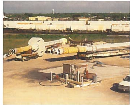
Three of the Horn Mountain truss spar's upper riser stems, one already fitted with its deck stopper assembly, prior to rail shipment.
