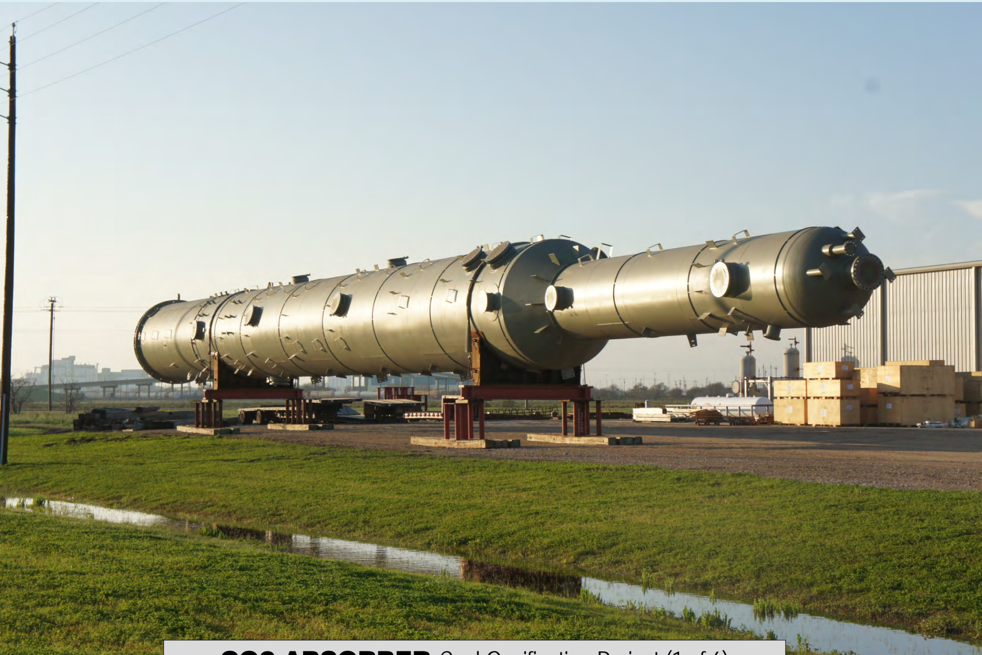
CO2 ABSORBER Coal Gasification Project (1 of 6)
