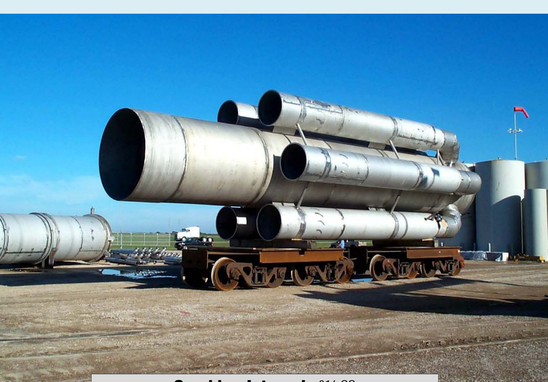
Scrubber Internals 316 SS
