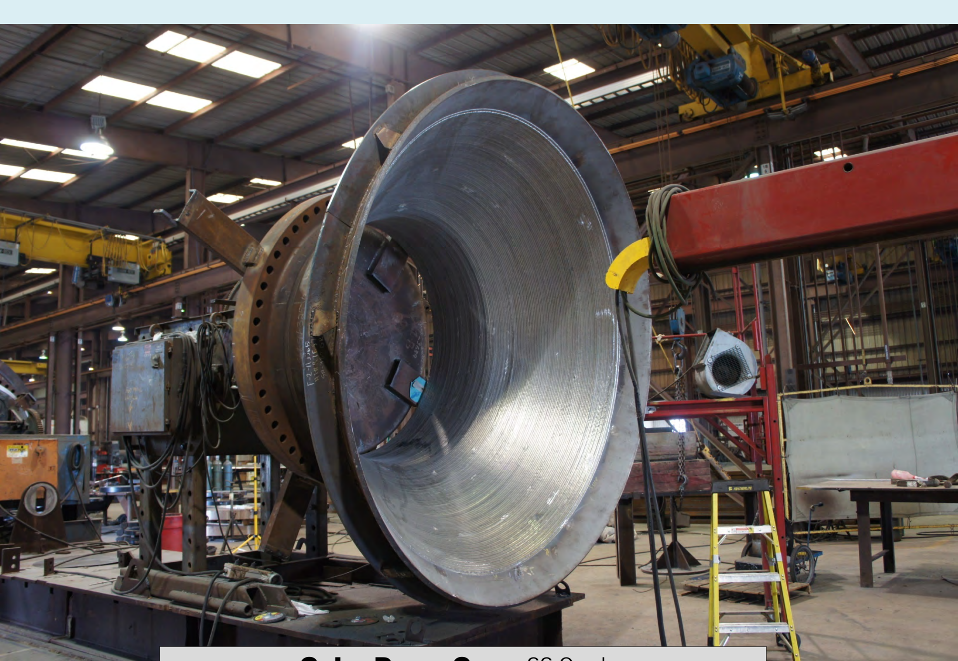
Coke Drum Cone SS Overlay
