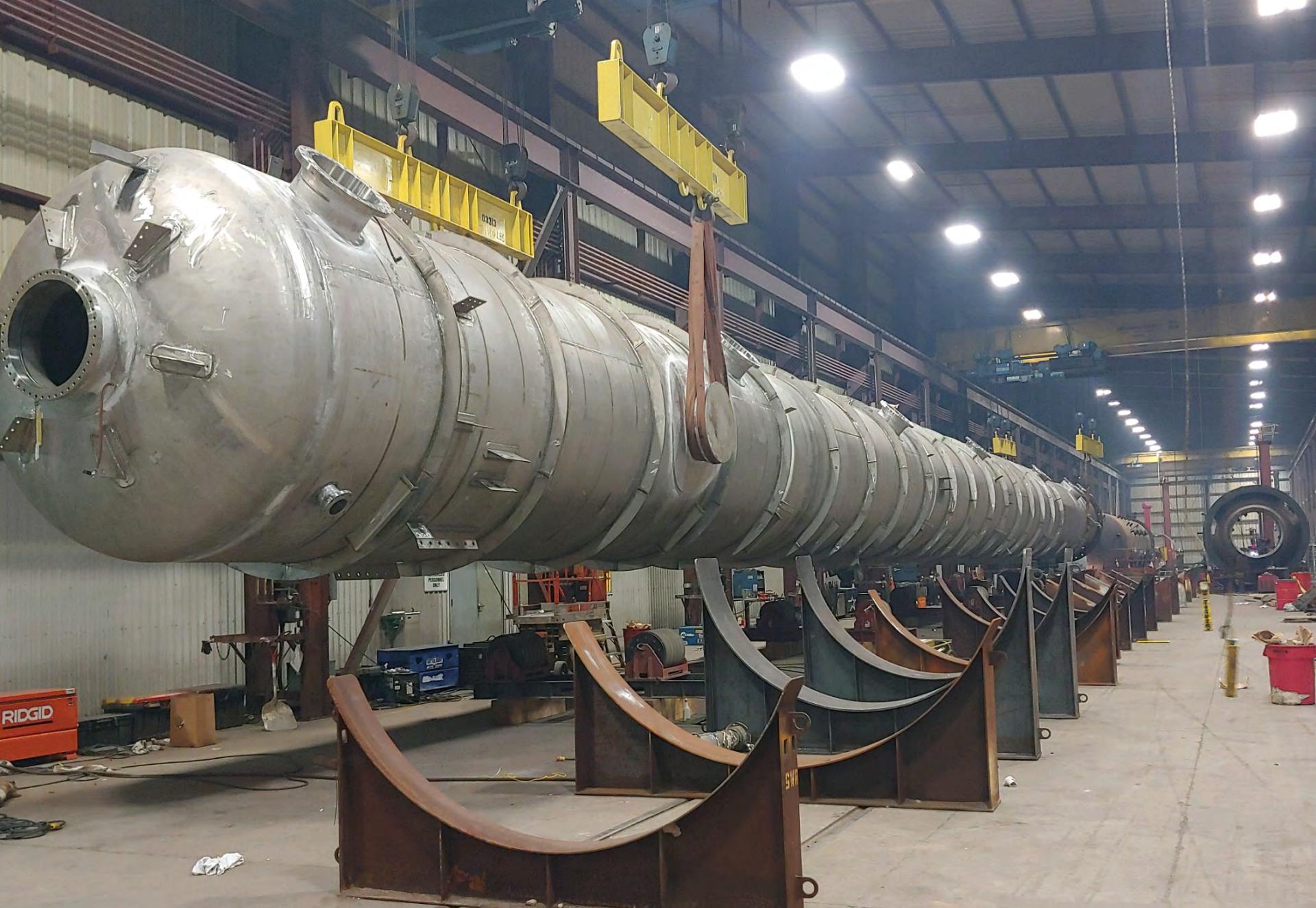
Shop Lift / Hydro Test: Hastelloy C276 Tray Tower
